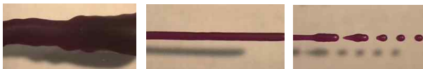
(a)overflow line (b)uniform line (c) Discontinuous line Fig. 3 Types of patterning line
