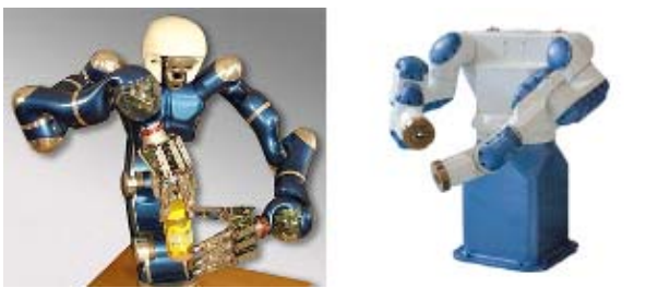
(a) DLR-LWR-3 (b) Yaskawa MOTOMAN-SDA10 Fig.1 Module Type Manipulators
