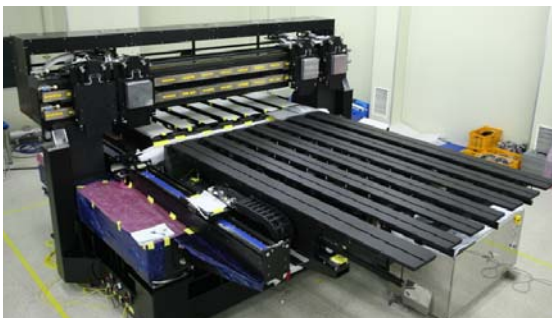
Fig. 1 A LCD manufacturing system with a XY positioning stage
