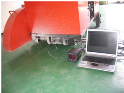
Fig. 1 Photograph of torque transducer equipped cutting M/C
