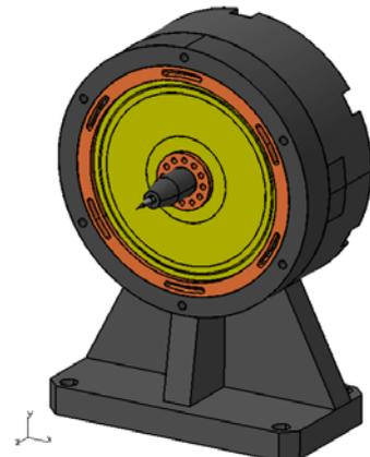
Fig. 6 Solid modeling of the diaphragm type OMM probe
