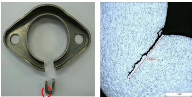
(a) Burring shape (b) Crack
