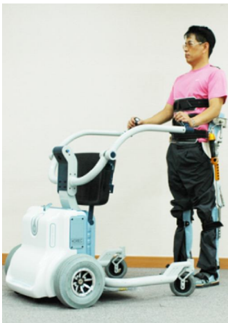
Fig. 1 Hybrid Gait Orthosis
