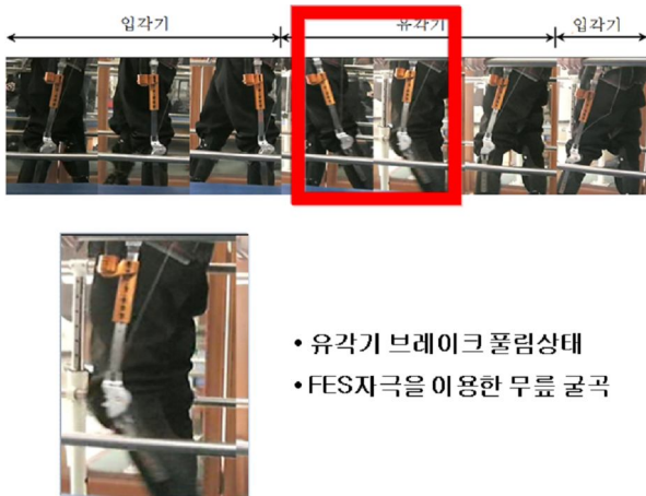
Fig. 4 Knee joint Flexion in Initial Swing Phase
