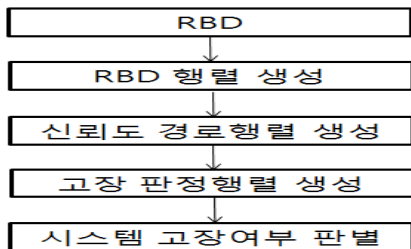
Fig. 3. The flow chart for a reliability calculation method of a system
