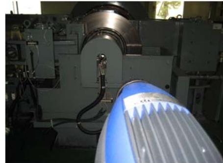
Fig. 1 Full-scale dynamometer and brake disc with high-speed infrared camera
