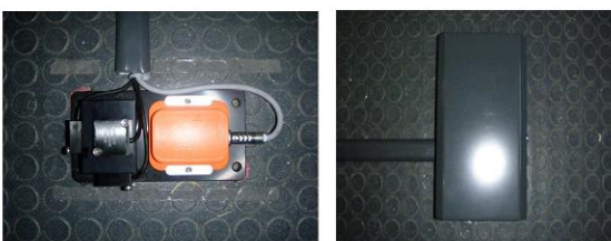
Fig. 6 Vibration accelerometers installed on floor of carriage 1
