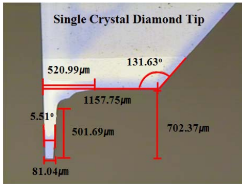
Fig. 3 Microscope image of single crystal diamond tip with width of 81.04 µm
