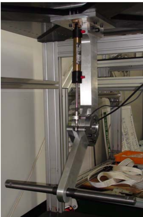
Fig. 4 One Joint System for Force Control Experiment
