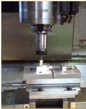
Fig. 4 Configuration of mandible bone sample fixture and tool dynamometer assembly set for implant drilling force monitoring
