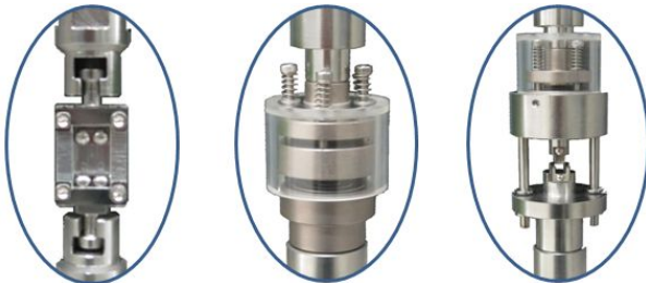
a. Tension b. Compression c. Bending Fig. 3 Grip & Jig for Material Tests
