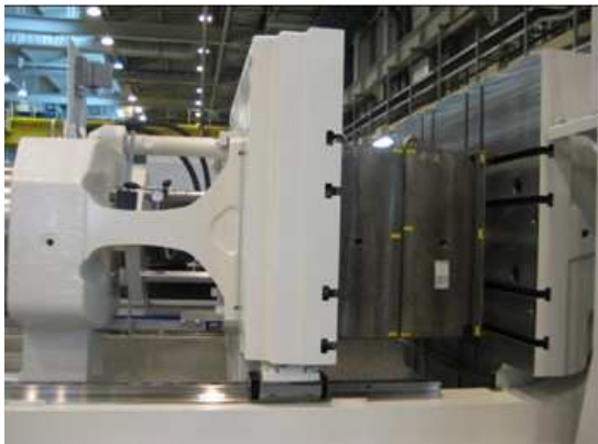
Fig. 5 Flex link elongation test equipment set-up
