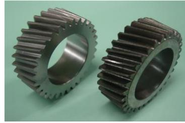
Fig. 6 Helical pinion made by hobbing and forging
