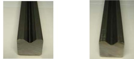
Fig. 9 Final drawn cross roller guide
