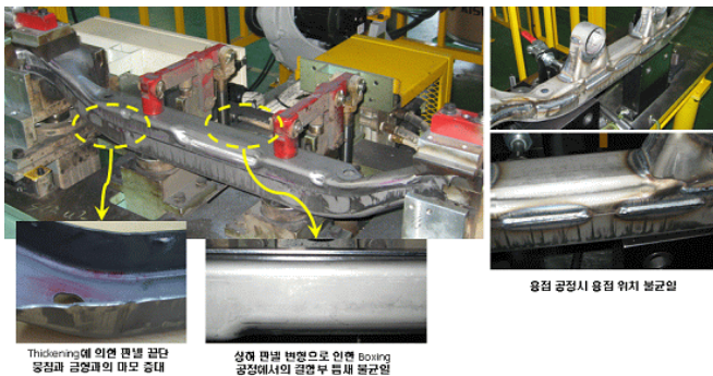
Fig. 1 Various problems in the boxing and welding process
