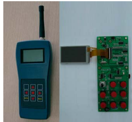
Fig. 6 Developed wireless controller
