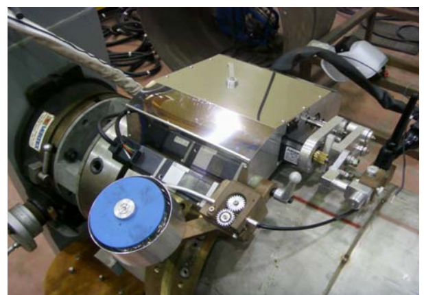
Fig. 2 Welding carriage and rail
