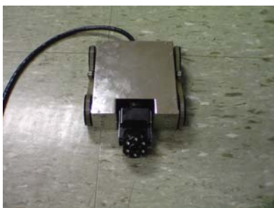
Fig. 3 Upper head inspection. robot
