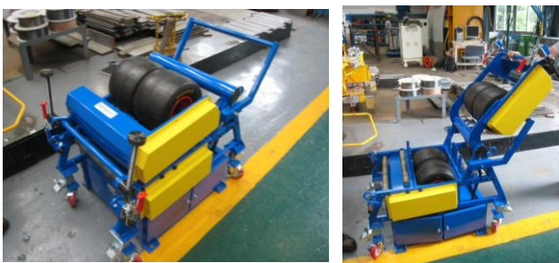
(b) DSME Co., Ltd. (Cable Pulling Feeder)
