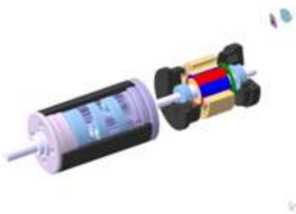
Fig.1 The actuator for robot (Gearhead+Motor+Driver)
