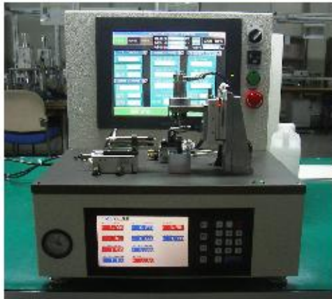
Fig 6 Measuring Machine by the LVDT Sensors
