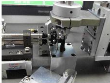
Fig 7 View of LVDT Sensors Part of Measuring Machine
