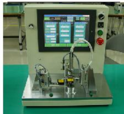
Fig. 5 Measuring Machine by the Laser and LVDT
