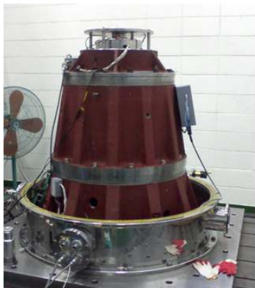
Fig 1. 5kWh flywheel energy storage
