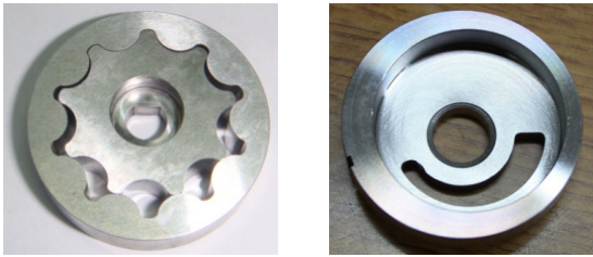
Fig. 1 Photograph of gerotor and cover plate
