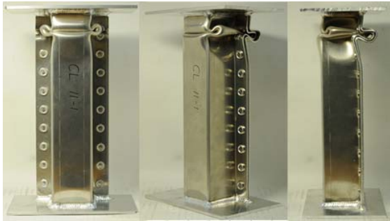
Fig.7 Shape of crash box using clinching after impact test (Exp.)
