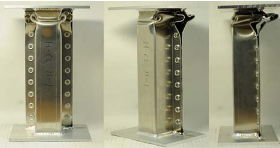
Fig.8 Shape of crash box using hybrid clinching after impact test (Exp.)
