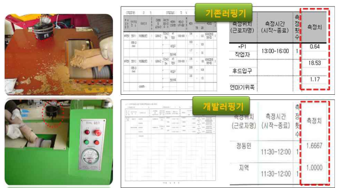
Fig. 5 The result of dust test at rubbing work area
