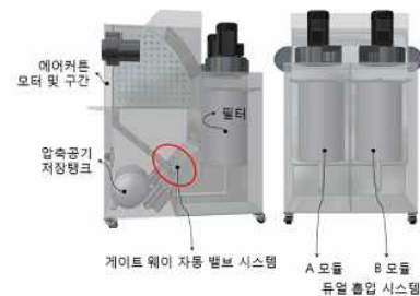
Fig. 2 Dual inductive mechanism
