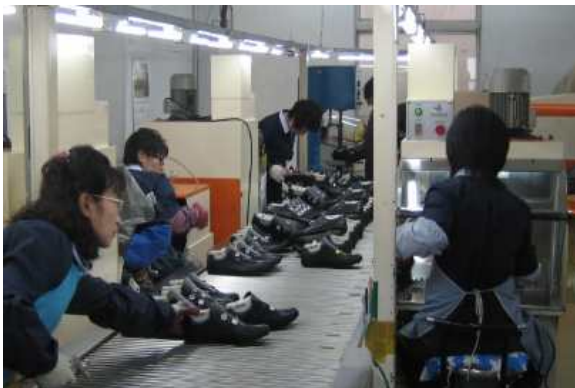
Fig. 1 The rubbing process in shoe factory
