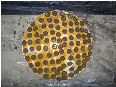
Fig. 5 A diamond-pellet tool for acquiring the radius of curvature
