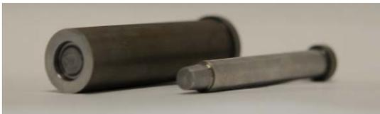
Fig. 3 Manufactured clinching tools with dimension in table 4
