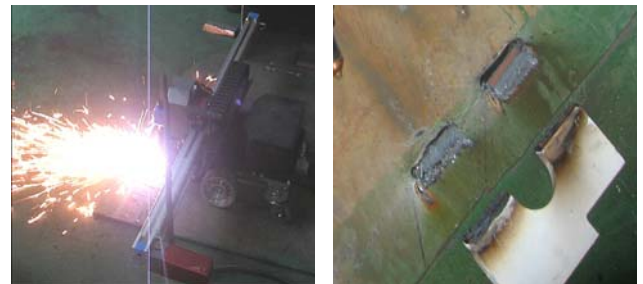
Fig. 7 Test and result of plasma-cutting
