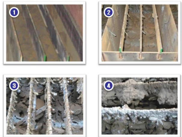
Fig. 1 The process of deposited-slag on steel-support
