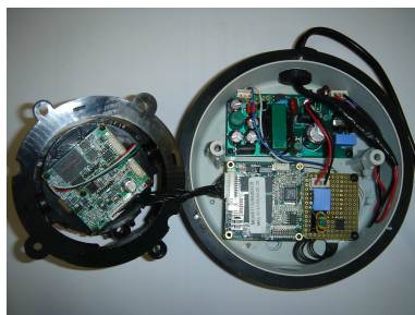
Fig. 6 Integration of modules inside PLC camera
