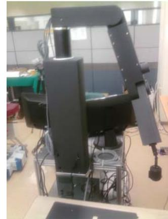
Fig. 1 Manipulator for Laparoscopic assist robot
