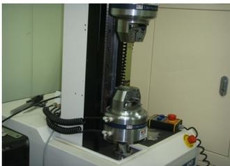
Fig. 1 Measurement of tensile strength of polymer films
