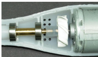
Fig. 7 Drive shaft connected with motor shaft by flexible tube
