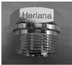
Fig. 1 Example of laser marking on mechanical part
