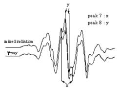
Fig. 1. Signal of alanine pallet irradiated with gamma-ray(1,500Gy) and mixed radiation measured with reference of Co-60(1,800Gy), showed ratio difference.
