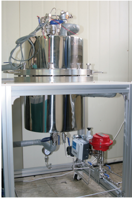
Fig. 1 Bench scale apparatus for hydrate production
