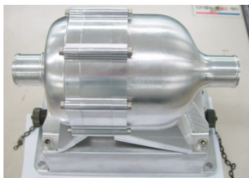
Fig. 10 Electric Water Pump
