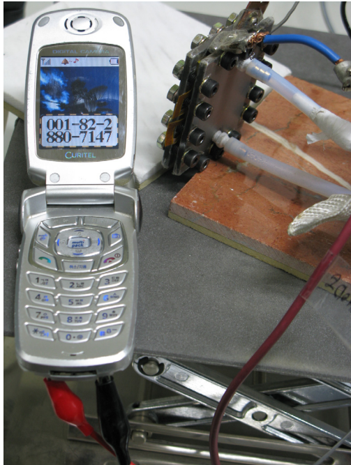
Fig. 7 Demonstration of the cellular phone powered by 6 cell stack PEMFC
