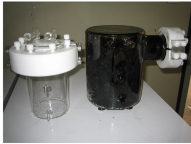
Fig.1 Lab-scale microwave waste tire pyrolysis reactor
