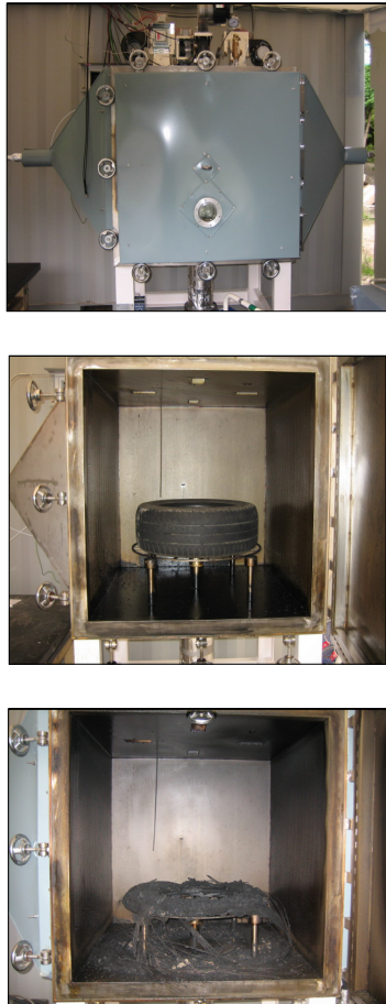
Fig. 2 Bench-scale microwave waste tire pyrolysis reactor
