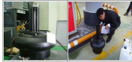
Figure 4. Performance test of fuel dispenser using standard cylinder
