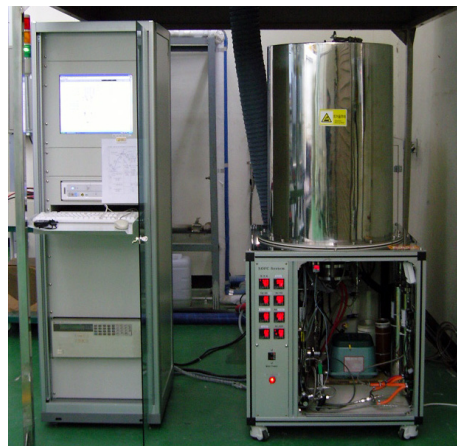
Fig. 3 1kW class SOFC system
