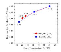
Fig. 1. Kerr rotation angle and Curie temperature of DyFe, HoDyFe and ErDyFe films. The angle of Kerr rotation was measured at the wavelength of 532 nm.
