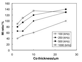
low frequency regime because the skin effect occurred at a low frequency in the case of electroplated wires with large core diameters.
