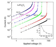
Fig. 1. I-V curves at various temperatures showing an electrically driven insulator-metal transition.
