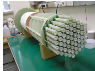
Fig. 1. Photograph of 61channel SQUID insert to measure biomagnetic field.
