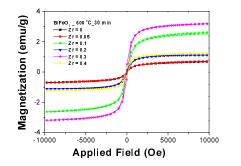
Fig. 1. The specific magnetizations of the  $BiF_{e_1,x}Zr_xO_3$ ; x = 0, 0.1, 0.2, 0.3, 0.4 samples calcined in air for 30 min at 600°C, as a function of field, measured at 20°C.
