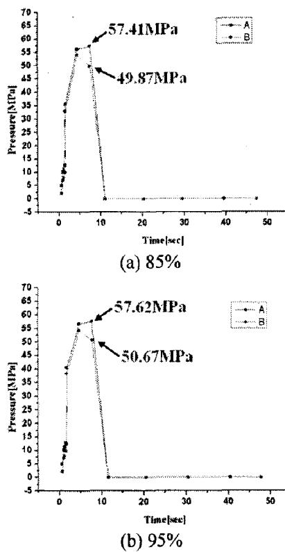
Fig. 3 Various cavity pressure profiles for velocity to pressure switchover
