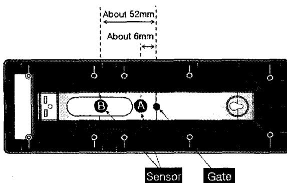
Fig. 2 Location of pressure sensors
