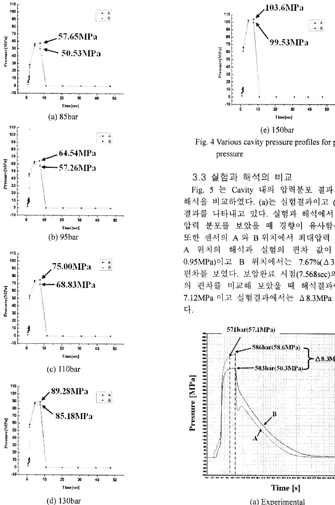
Fig. 4 Various cavity pressure profiles for packing pressure
