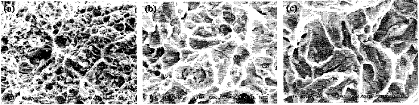
Fig. 6. FE-SEM fractographs of (a) no aged, (b) 550°C/1hr. aged and (c) 550°C/4hr. aged samples.
